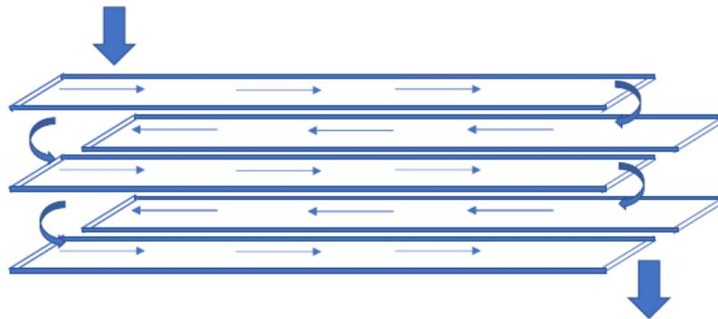
**Figure 3.** Operating principle of ModHeat dryer, © 2018 SFTec.
