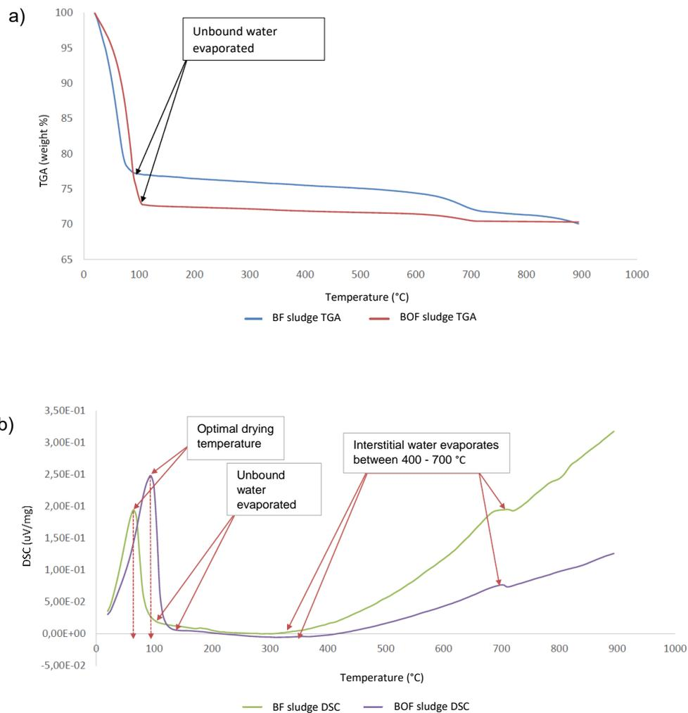
**Figure 7.** a) TGA -analysis and b) DSC analysis of BF and BOF sludge.
