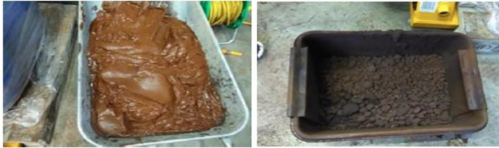
**Figure 8.** Converter sludge before and after drying, © 2018 SFTec.
